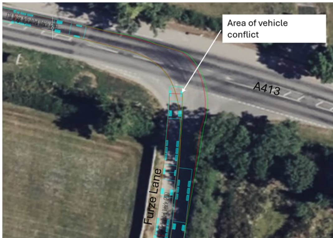
Figure 7: A413 / Furze Lane Junction HGV Swept Path
